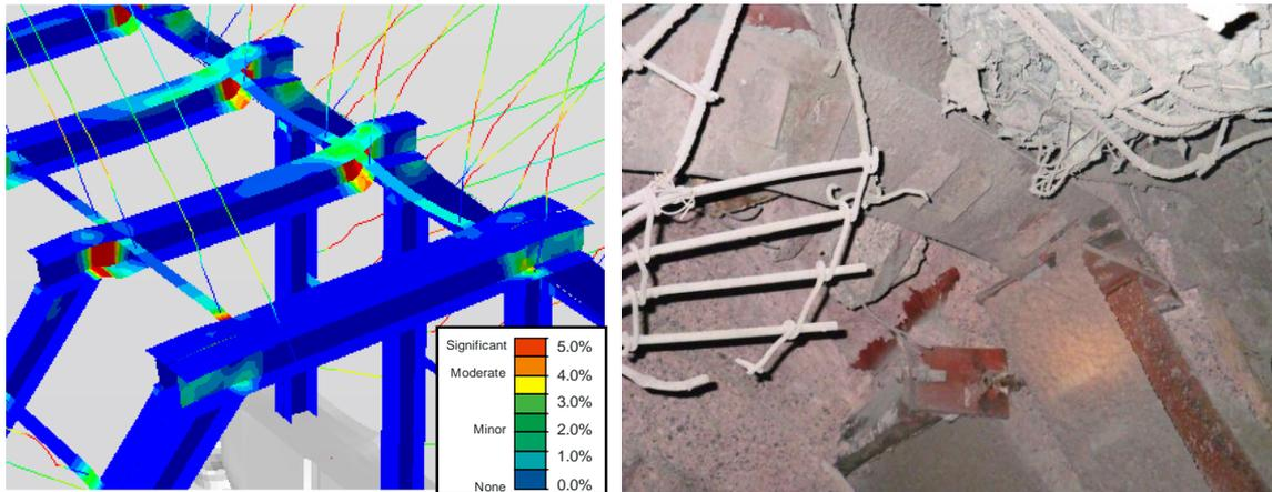
Figure 6. Example of steel set failure, and a close view of steel set failure in the model
