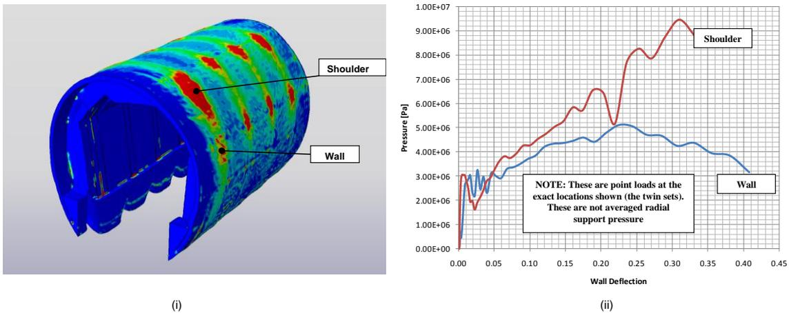
Figure 5. Simulated point loads versus radial deflection for the steel set design. These are not the average radial support pressures.
