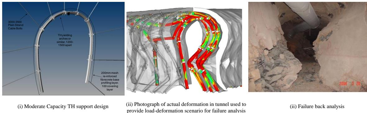
Figure 3. Simulated Shear Zone Support Damage, with 80MPa roadway
